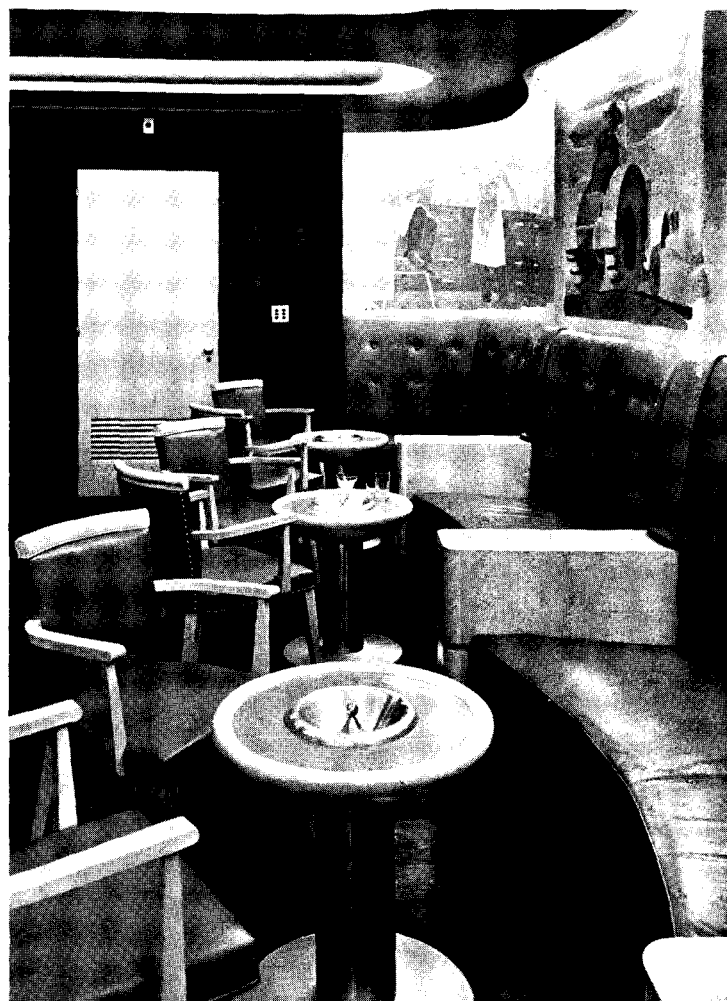
Totally indirect fluorescent lighting supplies all illumination.
