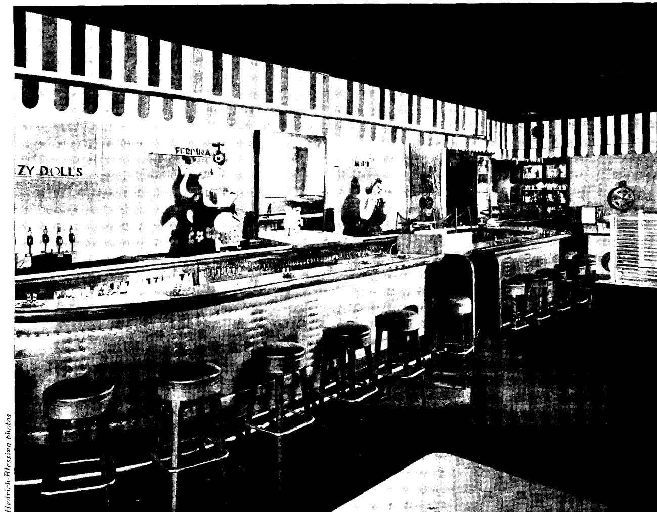
The gayly striped awning over the Midway Bar is of metal, and serves to mask the high-key lighting required both for display and for illuminating the bartender's work space.
