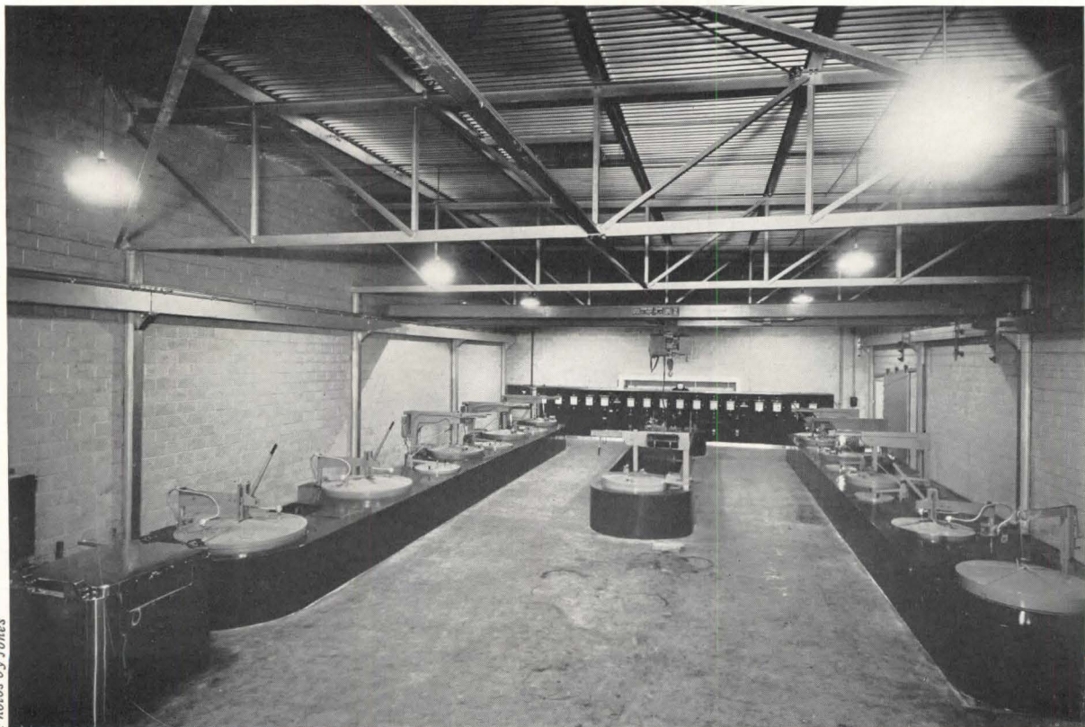
In heat-treat department, furnaces and cooling tanks are sunk in the floor for convenient access, and are serviced from basement rooms into which their lower halves project. Note controls at rear.
