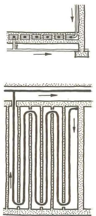
FIG. 23: Here air is heated in situ by pipe coils.
