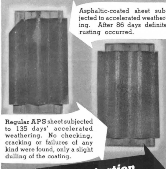
WEATHER-TESTED FOR EXTREMES — Here, in the Weather-Ometer, A P S panels were exposed to arc-light at temperatures up to 140°F., and then tested in cold-box at 10°F. below zero!
