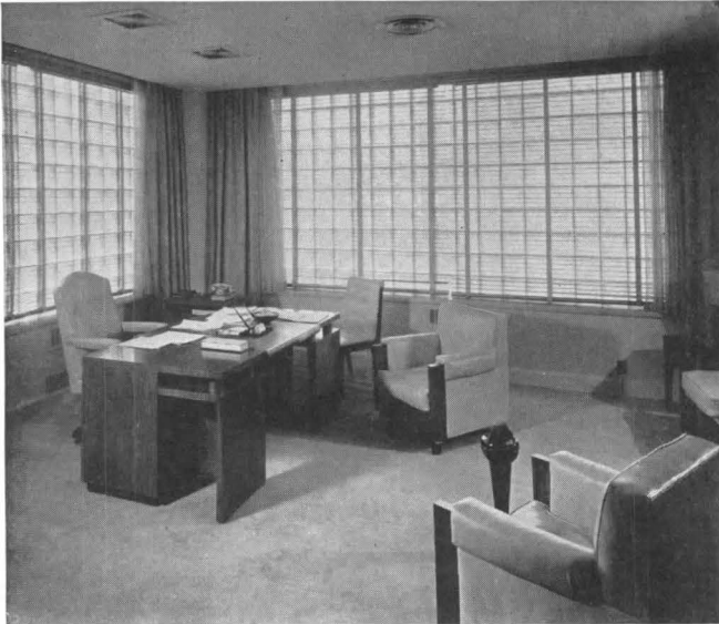
Executive office. Venetian blinds and draperies control the intensity of outside light flooding through the glass block. The ceiling is acoustic tile. Note air-conditioning outlets.
