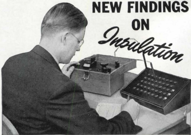
Taking temperature readings at 43 thermocouples with potentiometer.
