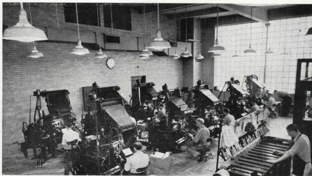
Linotype machines occupy one side of the composing room, with a space allowance for future additions. High-placed dome fixtures provide good lighting without any shadows
