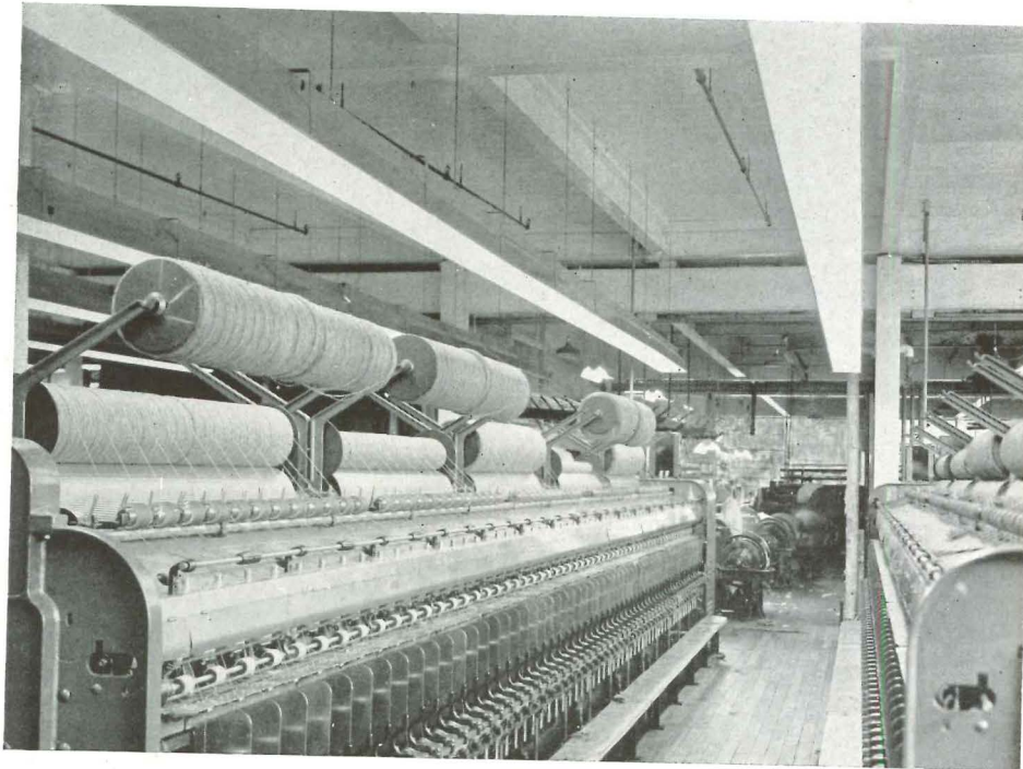
8. From the standpoint of seeing details regardless of their orientation, this lighting approaches that of outdoors in the shade. (Uxbridge Worsted Co.)
