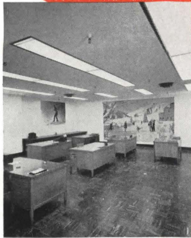
Illumination in the fourth floor General Offices averages better than 50 footcandles to increase efficiency, and provide unsurpassed working comfort for employees.
