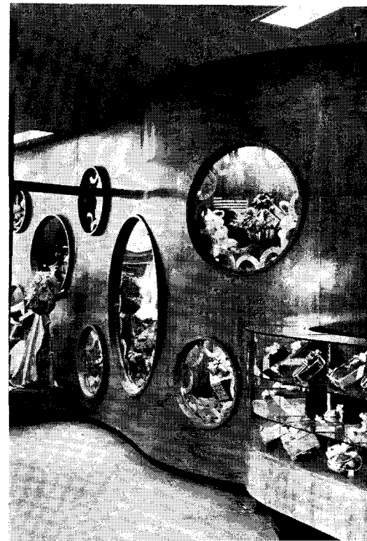
Right: Again the shadow-box idea, this time in a pattern of round boxes on the curving wall to catch the eye of entering customers. Since this wall encloses a traffic area, the boxes are recessed
