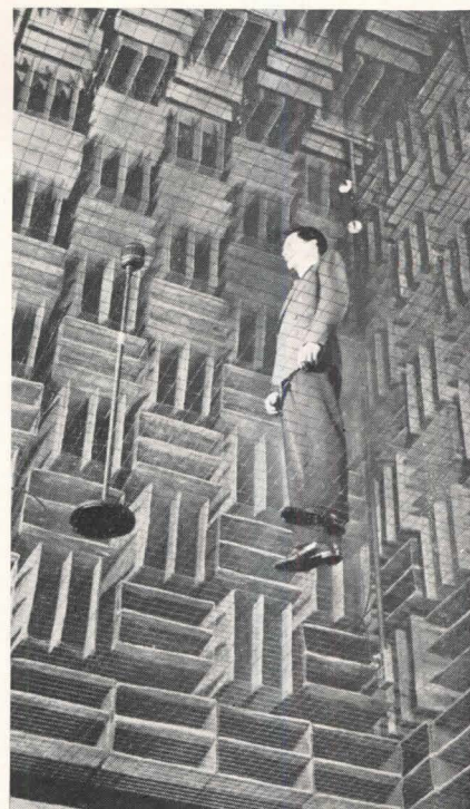
Special acoustical room is designed for complete sound absorption. Work floor is steel net suspended in space
