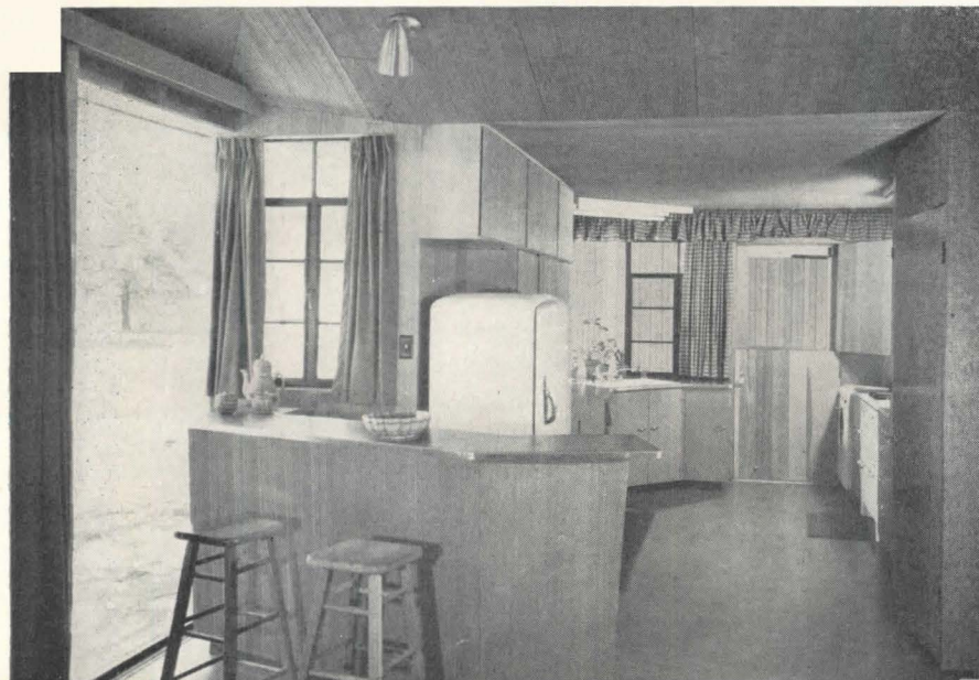
Left: breakfast bar is practically outdoors when sash is moved aside. Well-ventilated kitchen has divided door at end opening on breezeway. Floors are waxed red concrete
