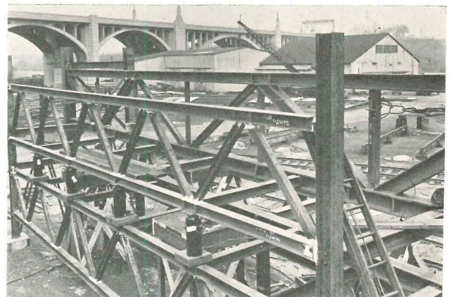
Above, one of the small laboratories. Below, the testing of the welded trusses before they were incorporated in the building. Note the hydraulic jacks between the pairs of trusses to produce the test loading to determine deformation (upper truss inverted to apply loading at same points as on lower truss)
