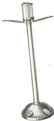
M-1030 Portable floor-type foot-operated dispenser. Delivers measured quantity of soap when treadle is pressed. Telescoping spouts swing horizontally.
