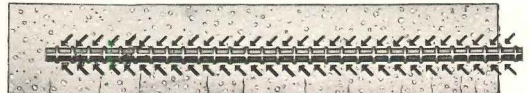
Laclede Multi-Rib Bars adequately transmit stresses to concrete by uniformly distributed anchorage. Small, closely spaced cracks do not open under load.
