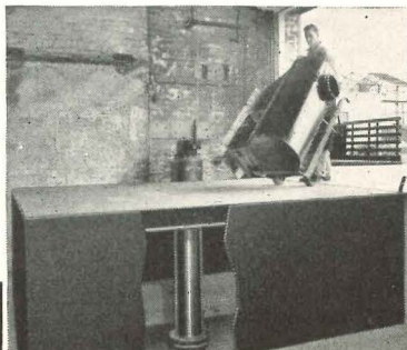
Ramps with Hinged Leveling Fingers and Throw-over Plate
