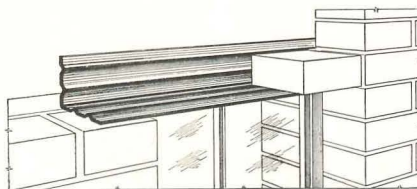
Pre-cut steel lintels save on-job labor
