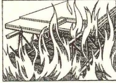
FIRE-RESISTANT because built of incombustible materials
