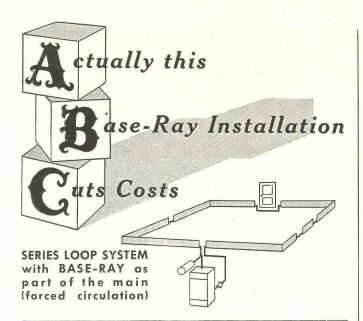
Study, for a minute, the diagram shown above. It tells the whole story. Installed in series, each BASE-RAY\* panel becomes part of the main. This can mean a saving in labor, pipe and fittings up to 50% of installation cost. In many cases, this saving is the determining factor in the landing of contracts. Further details on this Series Loop System, recommended by I-B-R, are given in their new Guide No. 5.
