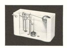
Interior view of Briggs Syphon Jet Closet Tank reveals latest design Anti-Syphon quiet operating flushing mechanism. This positive shut-off ballcock incorporates the latest type volume regulator, triple seal rubber ball, 1½-inch overflow tank valve, large refill tube and positive quiet action at high or low pressures. Every part quality engineered for lasting dependability.
