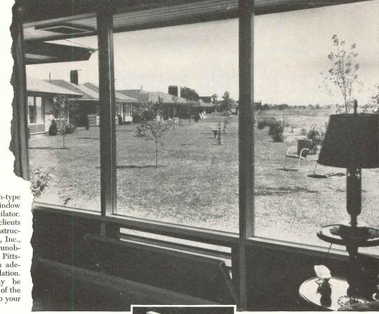
THE TREND in many ranch-type houses is toward a fixed window wall, with louver type ventilator. That's a feature which your clients will appreciate. For this construction, offered by Solar Air-Flo, Inc., Elkhart, Indiana, permits an unobstructed view through the Pittsburgh Twindow panels, with adequate ventilation and insulation. The louvered sections may be placed at top, bottom or sides of the Twindow panels, according to your design requirements.
