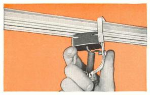
**To tap off power** at any point along the slot, simply insert twist-out plug and give it a 90° turn. Plugs are grounded on steel casing before contacts touch bus bars; narrow-access slot protects operator.
