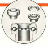
Exclusive Full-Jeweled Ball Bearing assembly consists of a movable and fixed raceway. When lateral thrust occurs, the movable raceway transmits the force directly to the bearings, which, in turn, are held firmly by the fixed raceway. Thus, the weight of the door is supported both laterally and vertically on ball bearings.
