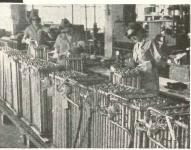
Attention to the many details that make up the completed unit typifies the Aerofin way. For instance, in this particular coil, careful brazing of the return tubes to the header plates assures leak-proof construction.
