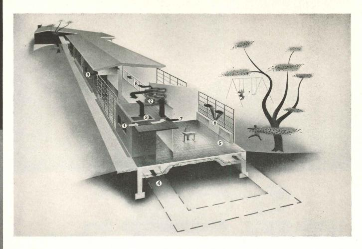
How the heating system operates: 1. Fresh air is taken in above exterior end door. 2. Air is drawn past steam heat coils by the fan. 3. Air leaves coils at 135F. 4. Air passes through concrete duct. 5. Air in duct keeps floor warm. 6. Air is thrown in front of cool glass area. 7. Half of air is recirculated (drawn from near ceiling). 8. Half of air is exhausted from classroom (drawn from near floor). 9. Air is exhausted to the outside
