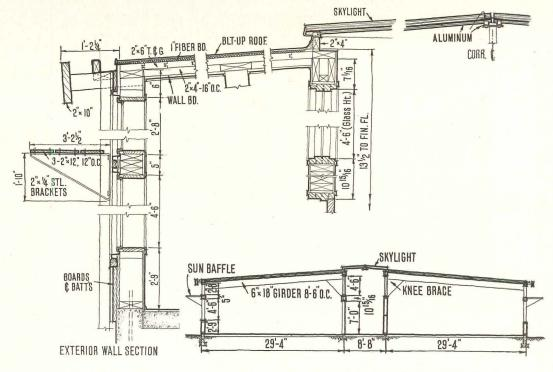
Section, details and photo show construction mostly of native wood, and method of borrowing light from interior corridor for classrooms either side. Each classroom wing will be a self-sufficient unit during normal school hours; only at recess, etc., will children have to use the outdoor, roofed corridors between wings
