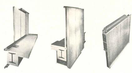
Illustrations from Stainless Steel Curtain Walls — A Progress Report On Methods: left, back and front of metal pan design combined with structural insulation; right, view of reinforcing-type textured steel facing, cast insulation
