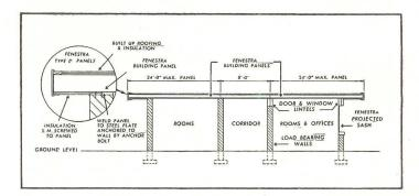
Interlocked Panels are simply welded to small plates mounted on top of concrete block walls.
