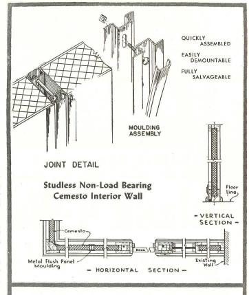
These details of interior walls erected with Cemesto Panels indicate the cost-cutting, space-saving simplicity which this modern marvel of building materials makes possible in all types of construction.
