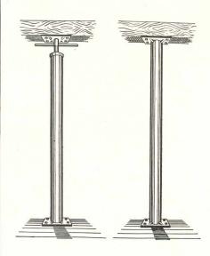
Plastic-covered columns are fabricated for either temporary or permanent supports
