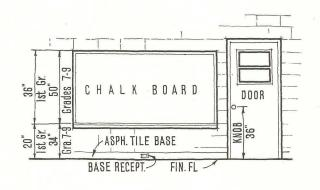
Typical classroom details. Above: section through washroom, with heights indicated for wainscoting, mirror and lavatory. Above right: heights of chalk board and door knob on typical wall elevation. Below right: arrangement of sink and wall cabinets
