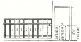
Typical classroom details used by Engelhardt, Engelhardt and Leggett. Left: built-in bench. Center: wall elevation with cork board and clock. Right: wall elevation with lockers, coat hooks and door. Height variations are indicated for different children's age groups
