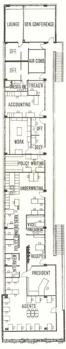
Framing-Reinforced concrete Exterior walls—Structural tile Interior walls—Plaster Floors—Asphalt tile Ceilings—Acoustic plaster Sash—Steel Store fronts—Aluminum
