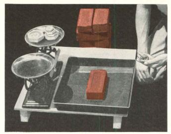
When placed flat in ¼-inch of water for one minute, a brick should gain not less than 5 grams (1/5-oz.) and not more than 25 grams (1 oz.)
