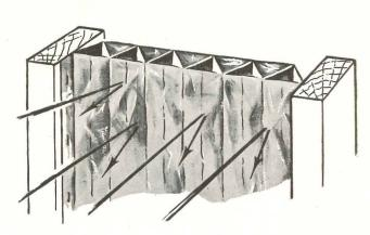
Tough aluminum is impervious to water vapor and yet has insufficient mass to extract heat from contacting air before reaching equilibrium in temperature with it. Colder air can support less vapor, and is an important cause of condensation.
