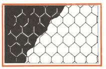
NOT SO SMOOTH, but much stronger, the right application of chicken wire reinforces both the asbestos cement and plastic weatherproofing finish.
