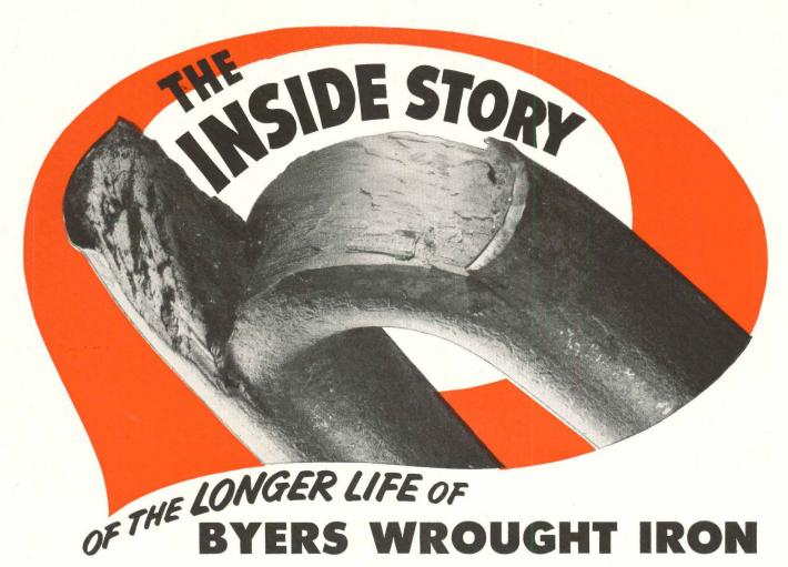
Every engineer will recognize this picture as a notch-fracture test specimen . . . and will appreciate the unusual physical properties
