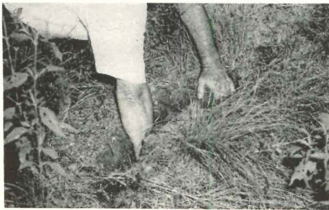
2. Crevices like this result from drying out of clay; enormous expansion follows when it rains
