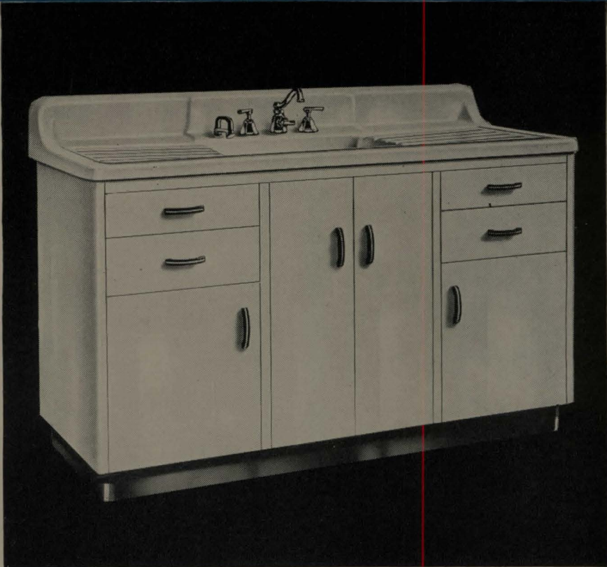
THE RICHMOND SERVILLA —Plate No. 1535: Double-drainboard roll-rim sink. Acid-resisting enamel. Drilled for deck-type supply fitting, with hose and spray. Sizes 54" x 25" and 60" x 25". Plate No. 1537: Sizes: 54" x 22" and 60" x 22".
