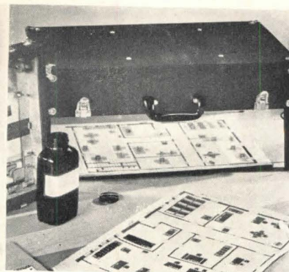
Left: artist places plastic cutouts on grid. Right: floor plan print is made in case
