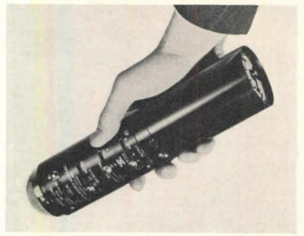
Small noise meter for field-testing runs on tiny hearing aid batteries
