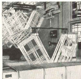
GALVANIZING. Assemblies dip deep into molten zinc, and come up with a heavy, smooth, uniform coating. Temperature and timing are automatically controlled with laboratory accuracy.
