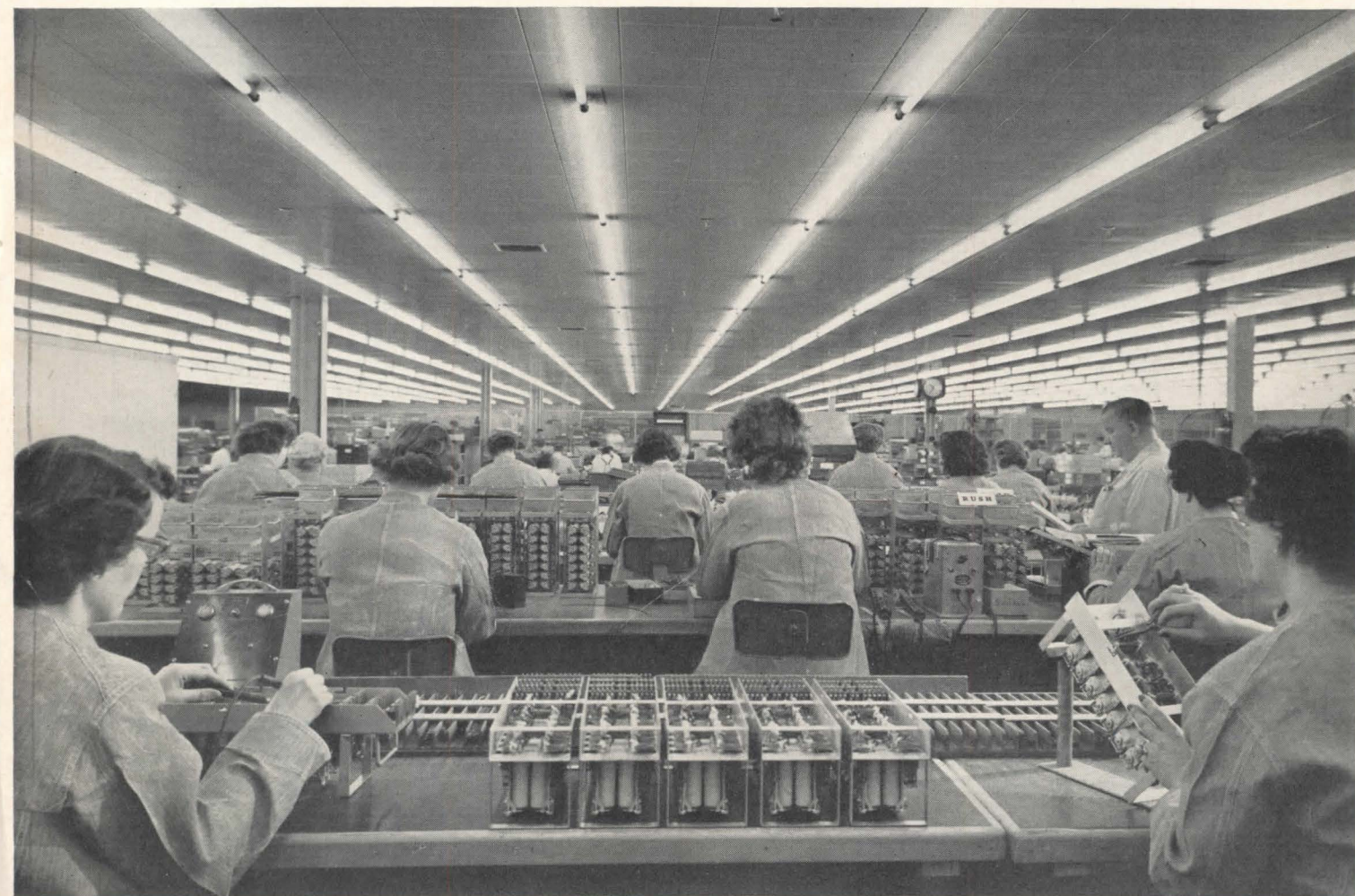
The 9-ft 3-in. ceiling, above, is finished with alternate panels of perforated metal acoustic tile or plain metal tile, with insulation between them and the roof joists to seal out dust from above. Typical office at right; the manufacturing area below
