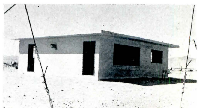
MASONRY BLOCK — Reinforced; 5 psi overpressure
