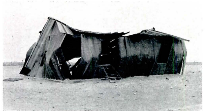
STEEL — Self-framing panels; 3.1 psi overpressure
