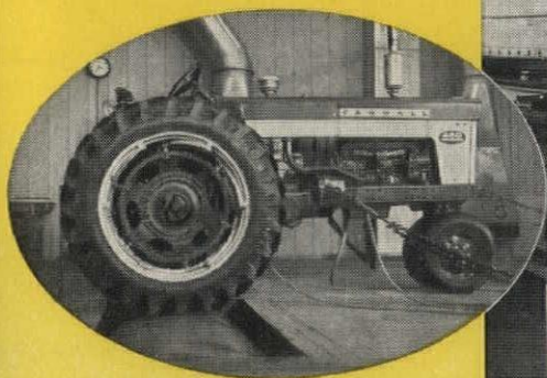
Undergoing an axle test, this Farmall Tractor #460 is secured on a Square D controlled treadmill.
