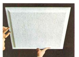
cost. Square lay-in panels are moulded in inverted coffer shape, projecting 2" downward into the room. As shown above, the visible surface has an attractive, low-relief, rippled texture. Panels are factory-painted white, but can, of course, be repainted to suit any decorative scheme. Measuring 24" x 24" x 2" deep and acoustically effective (NRC of .75) . . . Inverted Coffer Panels suggest interesting applications in supermarkets and other broad-expanse areas.
