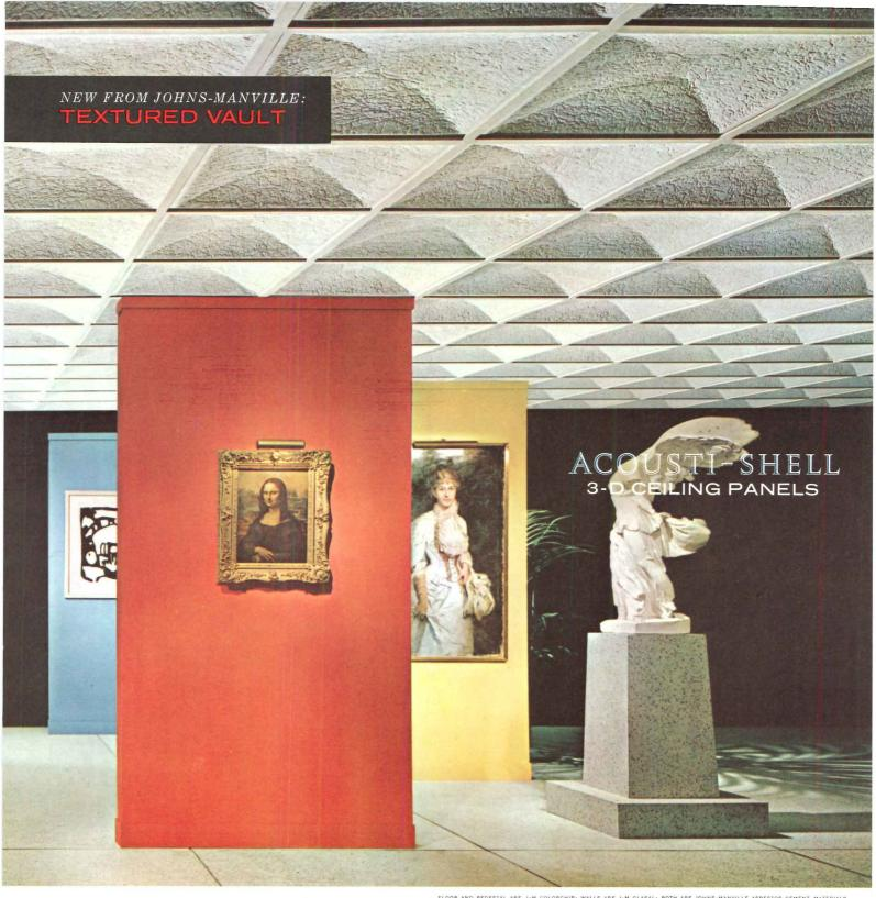
FLOOR AND PEDESTAL ARE J.M. COLORCHIP; WALLS ARE J.M. GLASAL; BOTH ARE JOHNS-MANVILLE ASBESTOS-CEMENT MATERIALS
