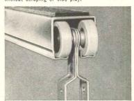
TROLLEYS—Foldoors feature a heavy duty trol-ley at every second hinge pair. This gives balanced weight distribution, adds to ease of operation and prevents sagging. Foldoor trolley pins are case hardened ¼-inch steel for extra strength.
