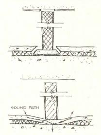
If partitions are set atop floating floor, either the topping will shear, or compressed topping and pad will offer direct sound path
