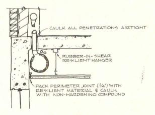
All penetrations must be caulked to prevent transmission of impact sound through piping, ductwork; also to stop airborne sound (above). Conduit and duct connections must be flexible to maintain impact noise reduction of floor (below)
