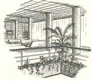
Used in, or adjacent to glass walls, round columns offer minimum obstruction to light and occupy minimum space for a brighter
