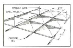
Installation of lay-in Textured Vault Panels is fast and simple in an exposed grid-type suspen-
