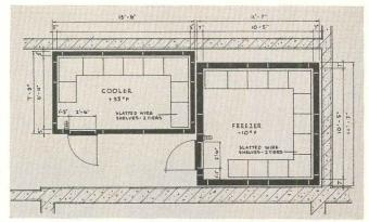
Plan view of two Walk-Ins, one a normal temperature and the other a low temperature, installed at **Dobyns-Bennett High School**, Kingsport, Tennessee.
