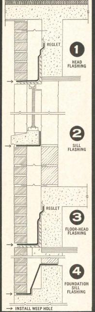
In cavity wall buildings, unsightly efflorescence and interior wall damage can result from accumulated water in the cavity. Causes: water penetrates joints in the outer wall; condensation forms on the inner wall.
