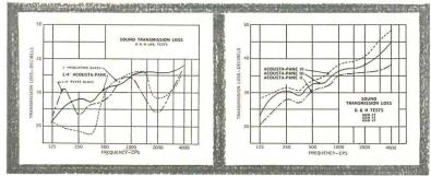
Acousta-Pane is especially effective in the critical frequency range for speech and normal office sounds—from 500 cps to 4000 cps—where ordinary glass is relatively "transparent" to sound.
