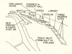
A new express highway parallel to the shore of the inlet, has been proposed by Aalto. Following the line of the existing rail approach, the highway will connect with large new parking areas covering the existing unsightly railroad yards. These garages will be covered with new shopping facilities. The diagram (left) shows the location of the cultural buildings planned for the site
