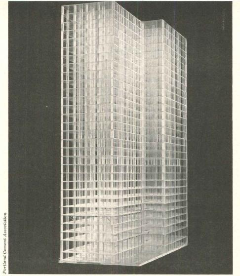
Housing in Chicago (Figure 4, left) indicated that 15 per cent less slab reinforcement was necessary than mathematical analysis showed. Also shear wall size and location was based on the structural model analysis. Cost of the model analysis was about 15 per cent of the savings it made possible.
