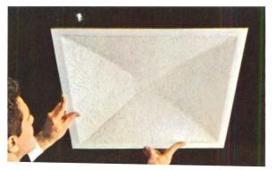
are moulded entirely of fiber glass with an NRC of .75. They are  $24'' \times 24''$ , rising gently to create a 2" vault. As you see above, the surface is made more visually interesting by a low-relief, rippled texture. White-painted at the factory for easy repainting if desired, Textured Vault Panels offer an opportunity to create a sense of height and elegance, as in the gallery above, and in larger institutional or commercial building areas.
