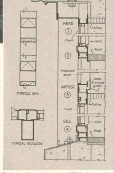
Typical wall section with LUPTON Curtain Wall
