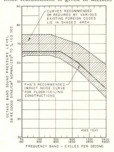
be caused by a vibrating appliance such as a dishwasher, toilet or food-disposal apparatus. The floor (or wall) is set into vibration by direct impact or mechanical contact, and sound is radiated from both sides of the floor. For this type of noise, the surface of the floor is very critical as regards the amount of noise generated.
