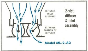
Air pattern controller, in both models, adjusts air flow a full  $180^{\circ}\dots$
