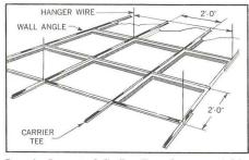
Lay-in Inverted Coffer Panels are quickly installed in an exposed grid-type suspension system
