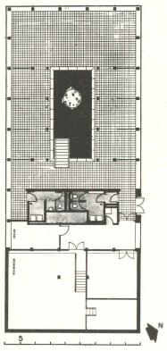
As the plans reveal, the upper level is set within a terrace for sculpture, while the lower level has a portion of its space devoted to wash rooms, office, storage and work areas. The entire building is air-conditioned, with specified humidity control to insure maximum protection for art treasures. The foot-deep pool of circulating water has a marble curb, a bottom of gray-black pebbles, and yields sufficient income from coin tossers to pay for its occasional cleaning!
