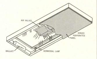
chamber is completely exposed to high-intensity rays emitted from the germicidal lamp and then evenly distributed into the room through perforated metal panels. The Pyle-National Co., 1334 N. Kostner Ave., Chicago 51, Ill.
