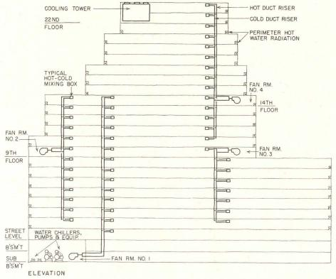
Simplified riser diagram shows that multiple fan rooms eliminate duct offsets
