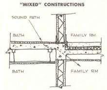
If different construction types are flanked, impact noise from the "poorer" construction will travel through structural slab on the floating floor side
