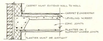
Plaster must be airtight to get most loss of energy through the structure and to prevent transmission of airborne noise
