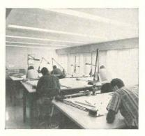
This office building incorporates the MAHONAIRE concept. Within the 7½" cells used for structural support were incorporated air distribution, troffer lighting, sprinkler system and acoustical treatment.
