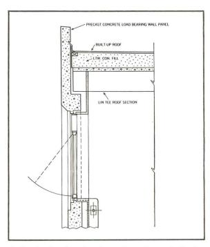
Section drawing shows how the prestressed concrete Lin Tees were connected to the precast load bearing wall panels with dowels (not shown) to eliminate all columns.
