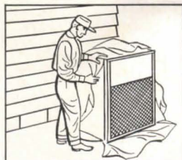
Cool-Air Chiller mounts outdoors; pumps refrigerated solution to cooling coil in Central-Air Unit; provides cooling and dehumidification.
