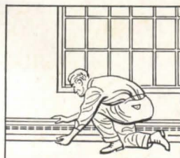
Smooth-Air Baseboard or Floor Drop-In Units distribute pre-conditioned warmed or cooled air . . . provide room-by-room heat control.
