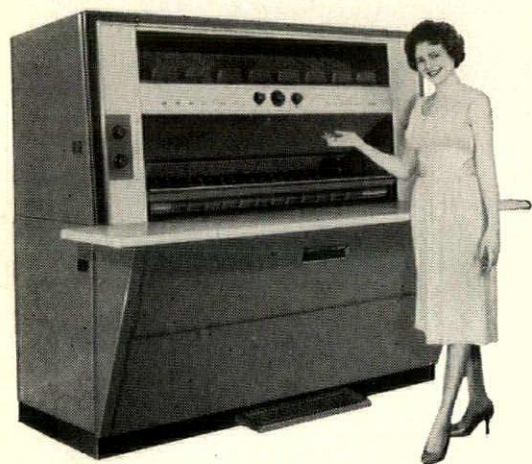
PRINTMASTER 900 ...accommodates materials up to 42" wide. Printing and developing speeds up to 75 ft. per minute. Just right for organizations requiring high quality copies at high production speed.
