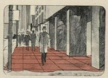
Snow Melting | Chromalox Electric Heater Mats and MI Heating Cable are embedded in concrete or asphalt sidewalks, driveways, ramps and steps to keep surface areas free of ice and snow. They eliminate manual labor and related costly agents such as salt, cinders and chemicals which often are tracked indoors to stain rugs and floors.
