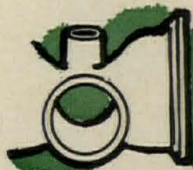
common vent (1) Saves chase space ...substantially re- duces the number of connections re- quired in a battery of toilets
