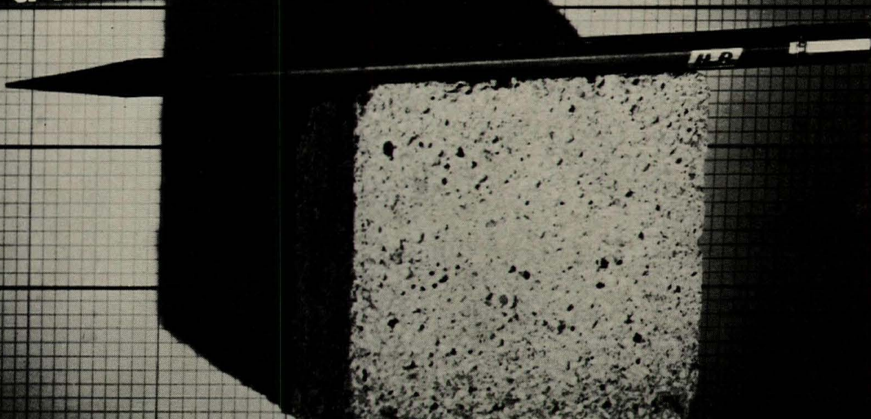
Actual size cube, cut from Permalite roof deck.
