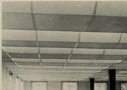
Armstrong B-48 Luminaire Ceiling System (4.8) All functions integrated into one unit—lighting, air distribution, acoustical control. 48" square modules, open both ends. One- or two-lamp fixtures, shielded or unshielded. 48" lamps each module, or 96" lamps running across each two modules (computer programmed for cool white). Vaulted modules combine with flat panels in any arrangement. (CU Range at Room Ratio 5.0, 30% Floor Reflectance, 50% Wall Reflectance: .75-.90)
