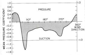
4 Wind suctions can create greater forces on a building than the wind itself, as can be seen in figure 4. This generally occurs when the wind makes an angular attack on the building. Figure 4 gives wind coefficients for only one point on a building model as tested in a wind tunnel.
