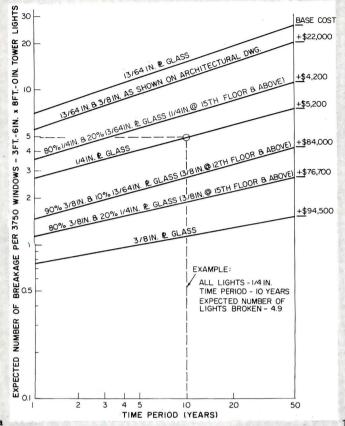
These two graphs illustrate how the risks and costs of glass can vary for a particular building (area and number of lights are fixed) as the thickness is changed. They also illustrate the effect of the variability
