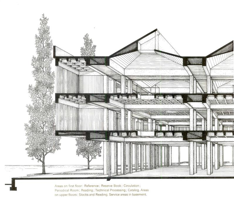
Double column arrangement sets up strong circulation patterns. Vistas of campus can be seen in all directions. Mechanical circulation handled between double column rows over circulation areas.
