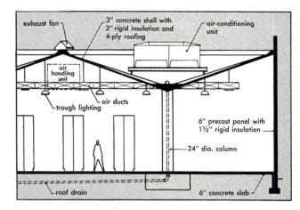
Design characteristics of the inverted umbrellas were fully exploited by fitting mechanical and electrical equipment into the cavities formed both on top and under the roof. This improved plant appearance on the outside. Inside, it saved 5 feet of headroom which would have been needed to house devices such as ductwork, fans, and air-conditioning units.
