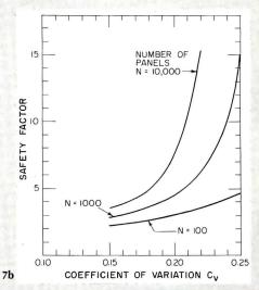
in the coefficient of variation do not have much effect, but with many lights, differences are great. With a high C<sub>V</sub> and a large number of lights, the safety factor becomes very high. Probability of no breakage in 50 years in figure 7a is 0.667; in 7b, 0.90.
