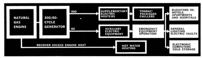
This air conditioning system provides a bonus of 60-cycle emergency standby power. Here's how it works. A dual frequency engine generator operates normally at 300 cycles for air conditioning. If main line power fails, an emergency transfer switch cuts in, and standby power is generated at 60 cycles. It's a power source that carries its own spare.
