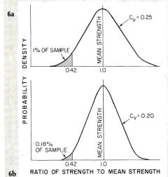
lights out of 1,000 would have a strength 42 per cent less than the mean. Figures 7a and 7b show how both the coefficient of variation and the total number of glass lights in the building change the required safety factor. With only a small number of lights, differences
