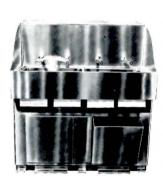
HOSPITAL SINK / A stainless steel surgical scrub sink has a pedal-operated spray bar that discharges thermostatically controlled water for an area of approximately 10½ by 8 in. There are pedal-operated self-contained antiseptic soap system, towel dispensers and towel disposal receptacles. Logan Hospital Equipment Company, Glendale, Calif.
