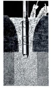
Diagram shows the lower end of a Vibroflot® machine in action to presettle sandy soil. Compaction is accomplished by a simultaneous saturation and vibration of the granular materials involved. During the application, fresh sand is added at the surface to compensate for the loss in volume caused by the increase in density (bearing capacity) of the compacted soil.
