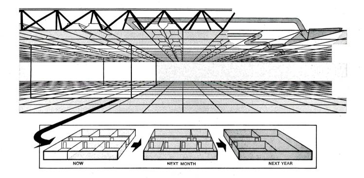
Here is a sea of space, air and light. And in this sea; heating, cooling, ventilation and illumination are furnished from above ceiling plane, in such dispersion that they do not restrict the possible arrangement of rooms. Then too—the structural system is so precise that by shifting movable partitions or operable walls, a great many room plan arrangements are feasible, present and future, while always providing environment matching or exceeding that with fixed partitions.
