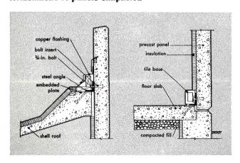
Panels were fastened to roof edge beams and the floor by bolting to steel angles which were welded to embedded metal plates. Inserts to receive <sup>3</sup>/<sub>4</sub>-in. bolts were incorporated into panels before casting. This made connections simple and expedient. And panels can easily be detached and relocated whenever plant expansion is called for.
