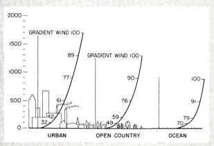
In open country the wind, obviously, will have faster velocities than in the built-up city. Graphs above (based on work by A. G. Davenport) show how the profiles of the wind vary with with the terrain "roughness."
