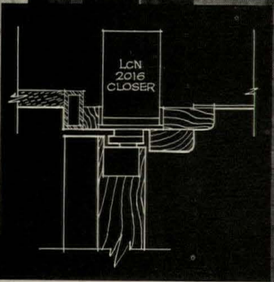
The LCN 2016 Closer is concealed in the head frame above the door. Arm disappears when door is closed.
