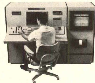
Standardized System 7 Selectographic Supervisory Data Center, with system analyzer and alarm printer module.
