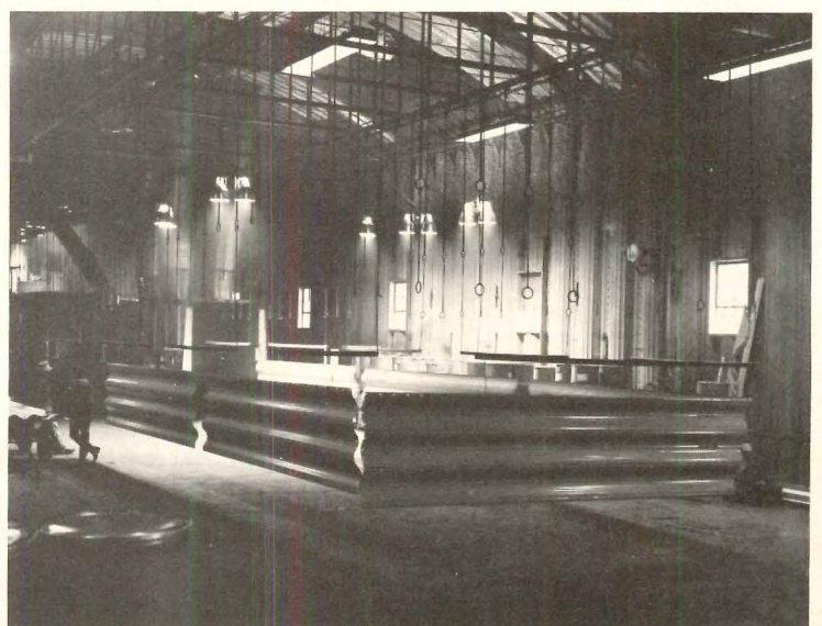
Galvanized steel panels pass through a multi-stage cleaning system and are primed before coating (top, left). Vertically reciprocating powder guns coat the panels and assure that all surfaces, including edges and joints, receive a uniform thickness (bottom, left). Coated panels are heated to 460 F in a tunnel oven so that vinyl powder melts and is fused to the substrate (top, right). Finally, panels are allowed to air cool (bottom, right).
