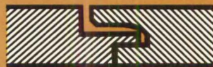
12" x 12" x 1/2" Self leveling tile for metal suspension systems, staple or adhesive application.
