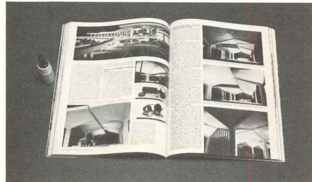
Effect of position of the light source in relation to the task on veiling reflections (at one time called reflected glare) is shown in these three photographs. In the top photo the light source (a bank of fluorescent lamps) is in front of the task, and the reflected image of the lamps is seen by the camera. In the center photo light comes from the left side, and in the bottom photo light source is to the rear of the task. Thus image of the lamps is not reflected toward the camera. The illumination from these two directions could be called "good footcandles."
