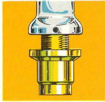
SQUARE OPENING Squared nipple fits into square hole in fountain top to prevent twisting and possible internal damage to cooler.
