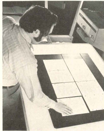
6. Pages of specifications are exposed eight at a time on a single frame of microfilm.
