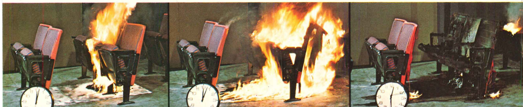
TEST TWO: HR POLYURETHANE containing flame retardants. Time: 1 minute, 30 seconds after ignition.
