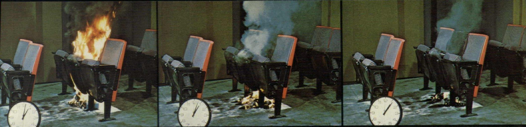
Major flames out. Time: 6 minutes, 00 seconds. Damage: 1 chair involved, fabric melting and smoldering on two adjoining chairs.
