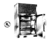
WM-CW\* series eye-level, wall mounted refrigerators are offered in 4 sizes featuring cold wall cooling systems with push-button defrost and automatic reset. Two removable, adjustable stainless steel shelves are provided. Front mounted grille removes
