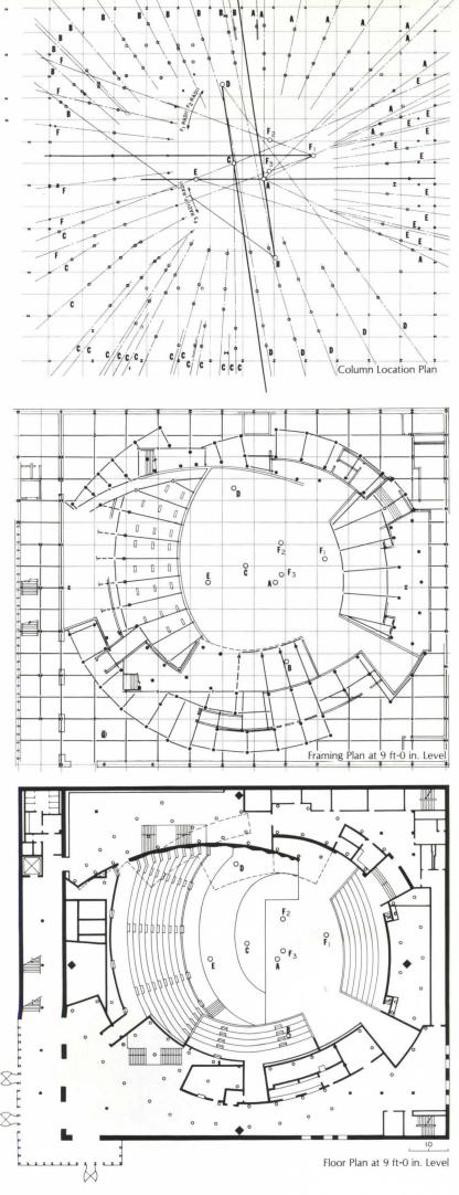
changes to an orthogonal-grid system with girders, beams and wide-flange columns finished square. The result of this expressed system change is definition of space and purpose: standing in the lobby and looking up or down through one of the several floor openings provided in the interface area, one is able to perceive both the location and extent of the hall space.
