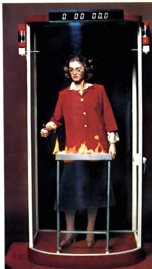
1. Flammable liquid ignited. Halon 1301 cylinders discharged.
