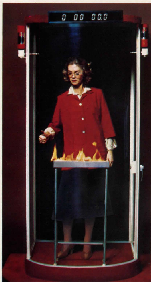
1. Flammable liquid ignited. Halon 1301 cylinders discharged.
