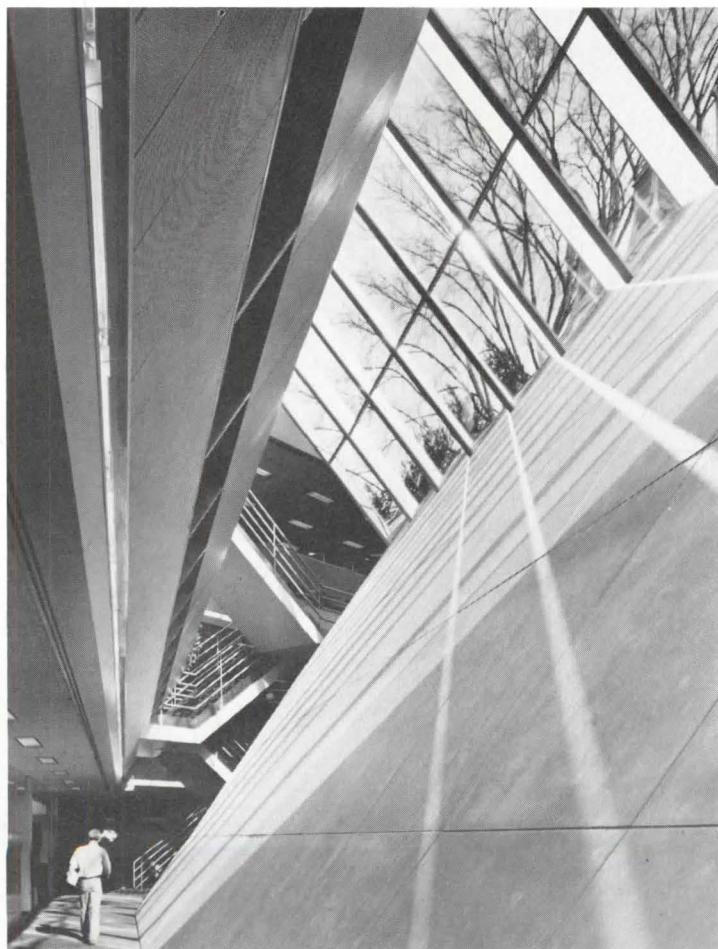
Reading desks set on stair railings take advantage of diffuse daylight from sloping glass (opposite). Skylight and mirrored baffles admit and reflect light to the bottom floor (directly above). The mirrors reflect outside views as well as viewers themselves (at top above).
