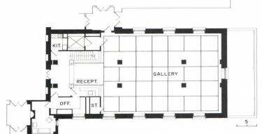
The versatility of the floating wall system is rooted in the ease of placing its 4- by 8 1/2-foot suspended sections at any point on the nominal 8-foot grid, including the diagonal. (Recessed locking devices firmly join the sides of adjacent frames, and bases are stabilized with hidden feet like those used to level household appliances.) But its virtuosity does not end with providing almost limitlessly mutable display
