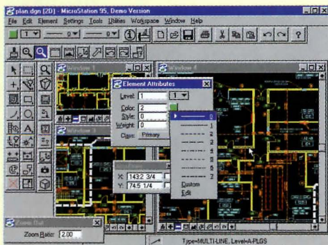
Selecting an element: With MicroStation 95, after selecting an element, you can then look at its attributes.
