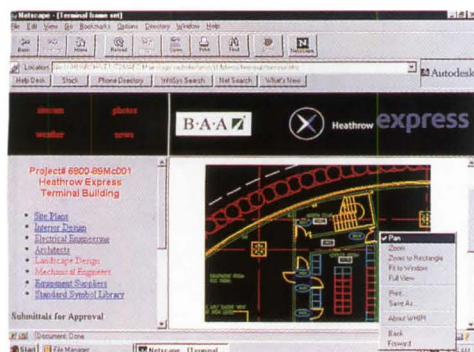
Viewing AutoCAD drawing in Internet project database for Heathrow. Note links to other items (at left on screen).
