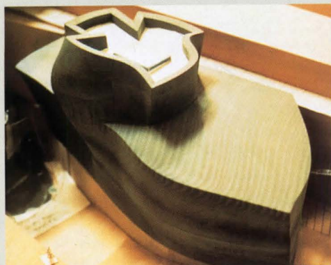
A COMPUTER-CUT MILLED MODEL IS MADE TO VERIFY ACCURACY
