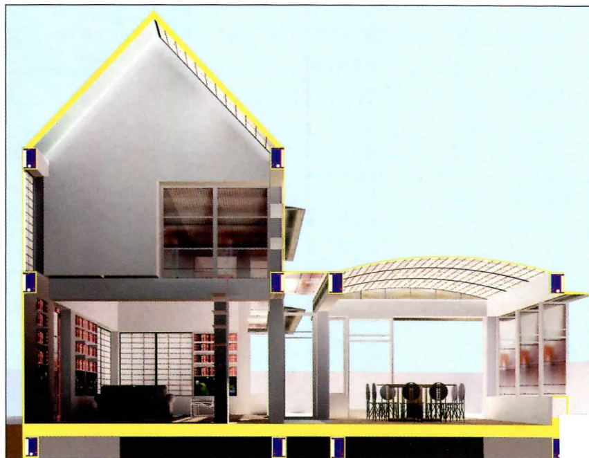
Single-family houses. MIT researchers are developing a Chassis and Infill component system (above) to replace conventional or panelized construction. The emphasis is on high-strength, high-performance, and lightweight new materials.
