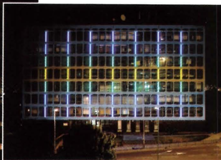
The facade lighting project incorporates 86 individually controlled, 10-foot-long cold-cathode tubes.
