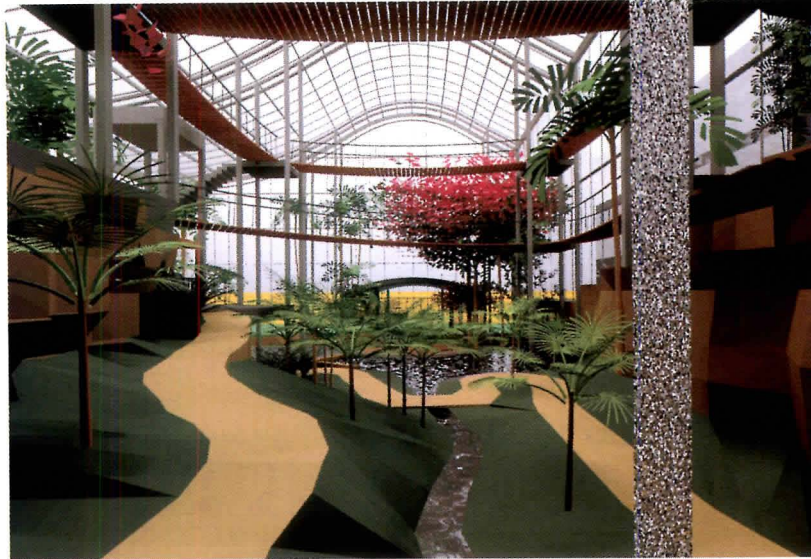
The Tropical Forest Building at the Phipps Conservatory lets in plenty of natural light for its permanent botanic residents. The simulation software Radiance was used to create this rendering of lighting conditions, and the results were used in the CFD analysis.
