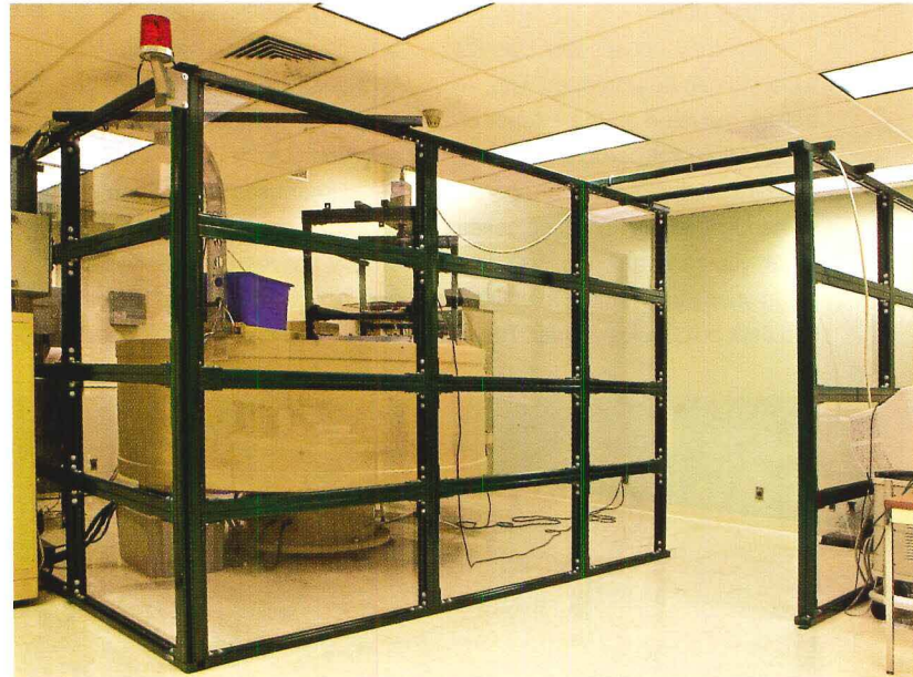
The centrifuge at the Department of Energy's Pantex Plant is protected by an enclosure made of the Unistrut structural metal framing system. The enclosure uses standard 4-by-8-foot polycarbonate bolted into U-channels.
