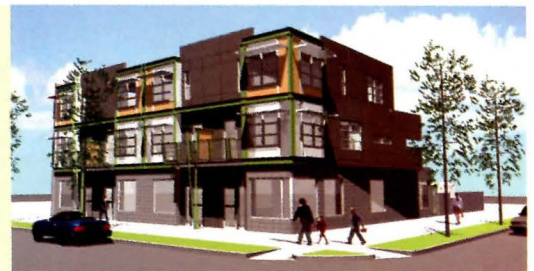
Using models created in Form-Z (left), Epstein showed clearly how the firm would transform a tilt-up concrete industrial building into office space with a new facade, more windows, and a glass corner.
